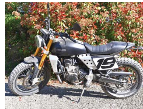
Flat Track variant runs 19-inch rims at each end, with road tyres and modified styling.
