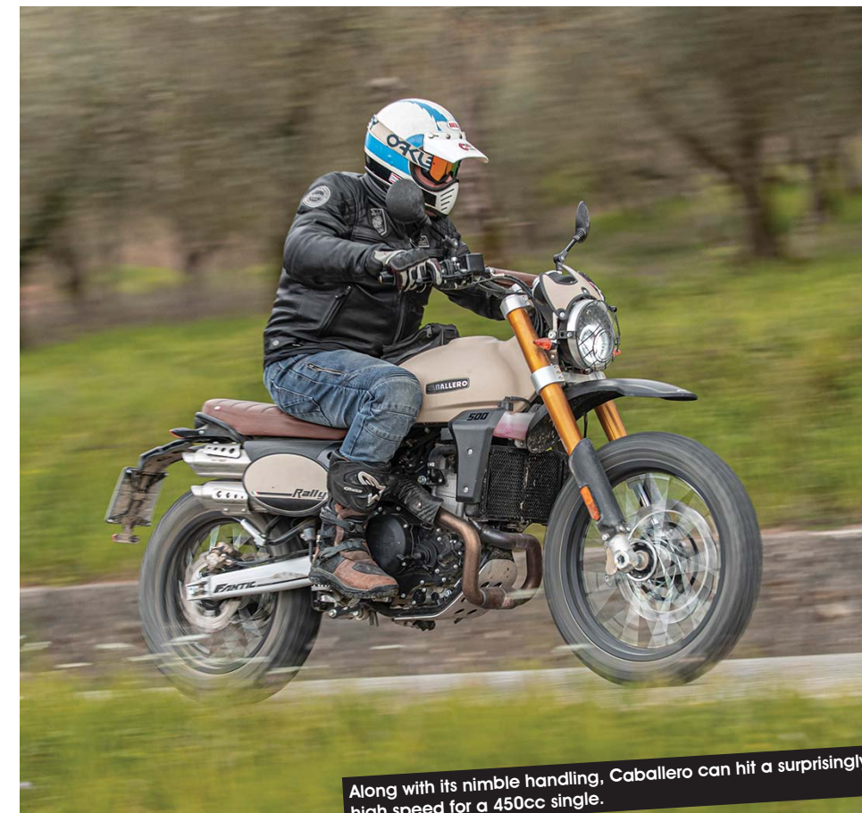
Flat Track variant runs 19-inch rims at each end, with road tyres and modified styling.
